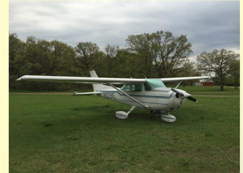
N8291E is a 1979 Cessna 172N. Known as the Skyhawk, it is the world's most common general purpose and training aircraft. A 160HP engine allows for a cruise of 105knts. Gross weight is 2400lbs with about 900lbs useful load. 40 gallon fuel tanks give 91E a 400 mile range at a comfortable 9 gal/hr. The avionics package features dual flip-flop NAV/COMMs, ADF, DME, and a VFR GPS. 91E had a new interior in 2005.
