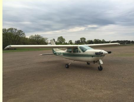
N122WR is a 1975 Cessna 177RG. Known as the Cardinal RG, it is a cross country dream come true. A 200HP fuel-injected engine and retractable landing gear allow for a cruise at 140knts. Gross weight is 2800lbs with about 1000lbs useful load. 61 gallon fuel tanks give 2WR almost a 900 mile range at a comfortable 10 gal/hr. The avionics package features a Garmin 430 GPS/NAV/COMM, S-Tec 2 axis Autopilot, DME, engine analyzer and a fuel monitoring system.
